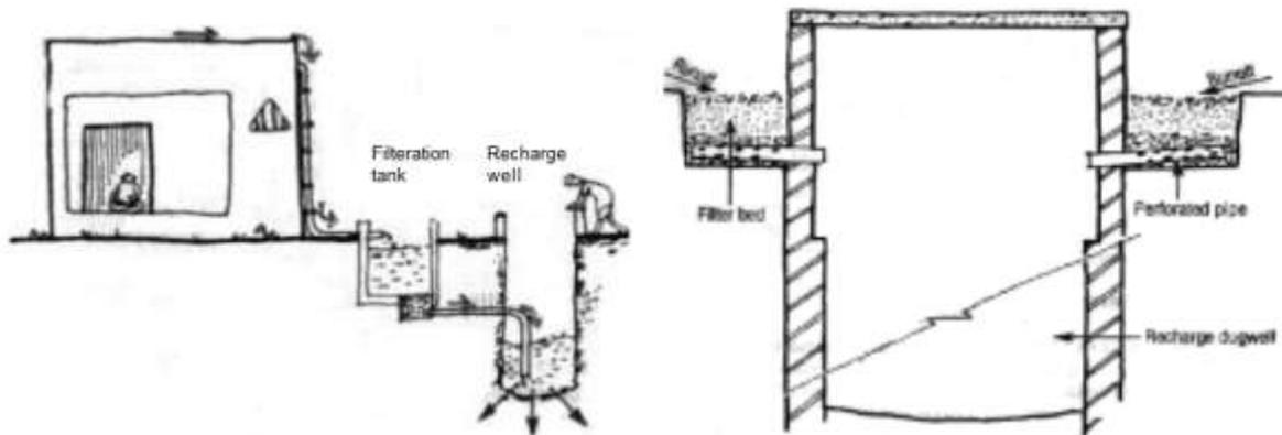
Fig. 6 Simple diagrams showing roof-top rainwater harvesting and surface run-off harvesting
