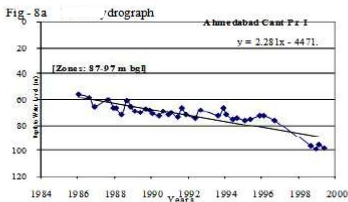
Fig. 3 Graph showing Depleting ground water levels in Ahmedabad
