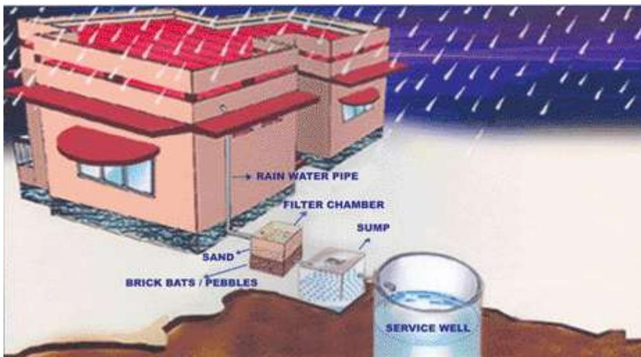
Fig. 10 Rainwater Harvesting at individual level
