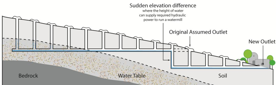
Figure.2 Schematic section of a sudden elevation difference (drawn by the author)
